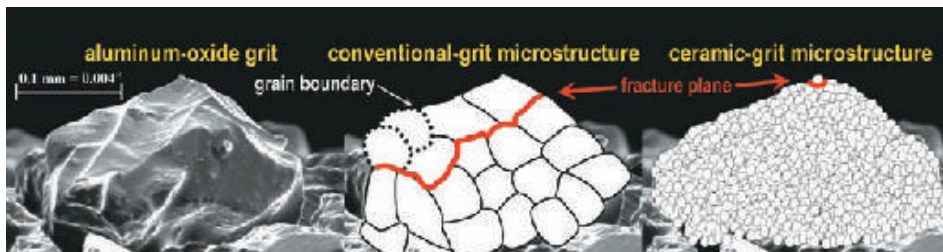
A ceramic grit fractures into smaller pieces than a conventional Al_2O_3 grit.
