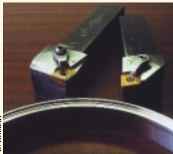
Stellram's SP4036 insert, with the new 3J chipbreaker geometry, helped Voss simplify the machining of a tough aerospace alloy.
