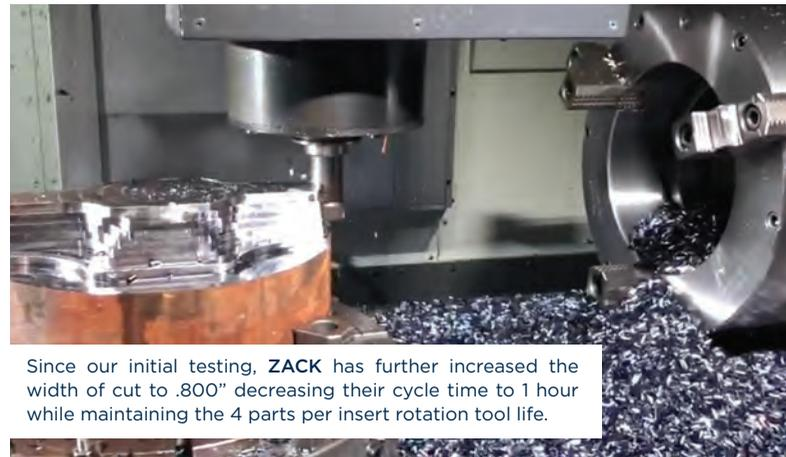
Since our initial testing, ZACK has further increased the width of cut to .800" decreasing their cycle time to 1 hour while maintaining the 4 parts per insert rotation tool life.
