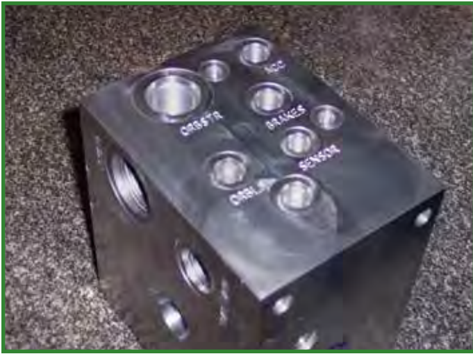
An example of one of the many deep-hole drilling applications performed at Anderson using the Walter DC170 drill.
