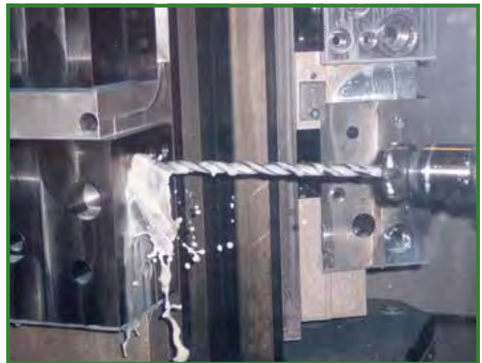
The new Walter DC170 drill in operation at Anderson Machining Service drilling one of the many holes in a manifold.
