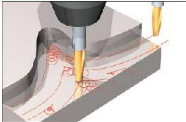
The trochoidal milling technique involves moving the cutter in radius paths as it cuts, rather than in a straight line. The circular toolpath minimizes tool engagement, aiding in the cooling of the cutting edge, and makes side loads on the cutter lighter and more consistent.
