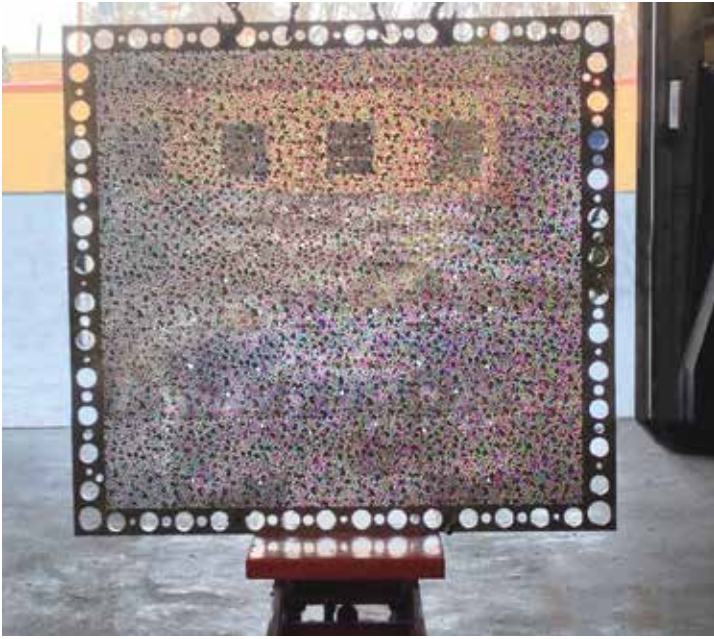
The 27,000 holes that are drilled into both the punch pad and stripper plate for the fiberglass tile creates an almost translucent appearance.
