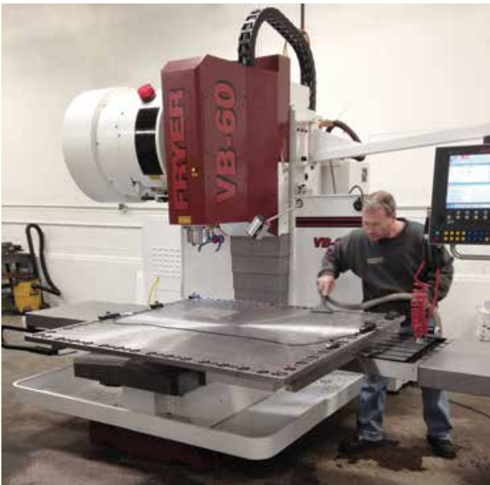
Toolmasters Inc. was able to reduce cycle time necessary to drill a punch pad and stripper plate for an architectural application by adding Walter Titex drills and a Fryer VB-60 machining center.
